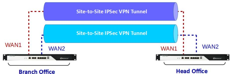
Figure 4: IPsec VPN Tunnels Termination and Load Balancing
