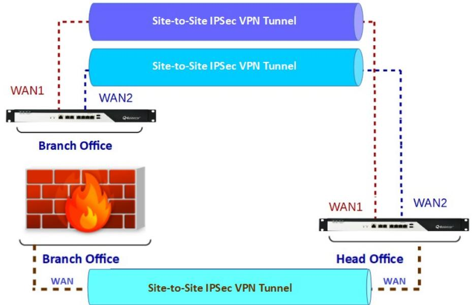
Figure 5: IPsec VPN Tunnel Termination on Q-Balancer & Firewall
