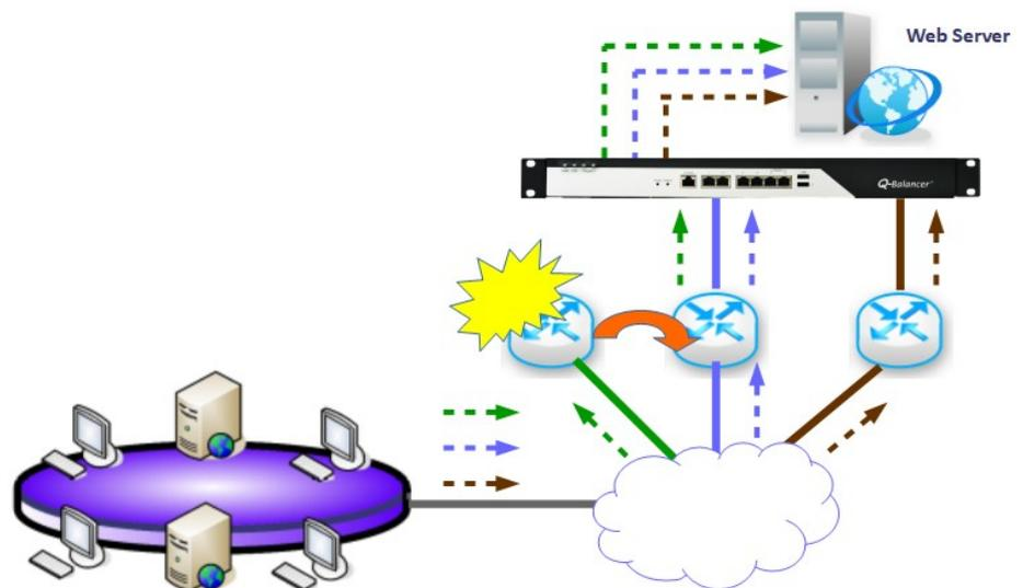
Figure 2: Inbound Load Balancing
